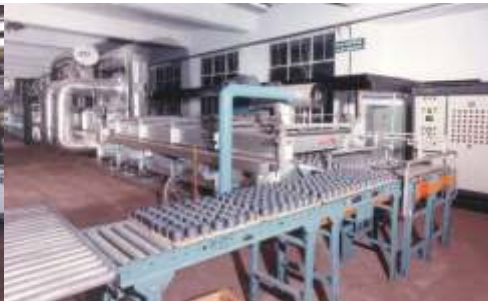
Roller Hearth, Gas fired 75 metres long, world scale sintering kiln.
