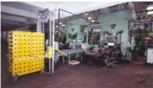
200 and 300 T Hydraulic Presses with automatic pickup and retrieval.
